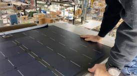
**IMPORTANT:** Strokes for the squeegee should start in the center of the panel and move at an angle toward the edge and the remaining release liner.
