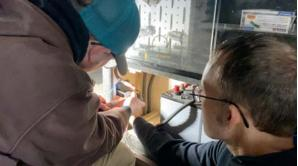
Remove the fuse in the wiring harness going from the charge controller to the battery.
