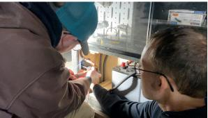
Remove the fuse in the wiring harness going from the charge controller to the battery.
