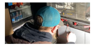
Measure the battery voltage to confirm 12V correct polarity, and reinstall the fuse.
